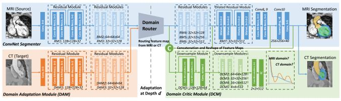
Figure 2: Overview of our proposed plug-and-play framework for cross-modality domain adaptation. The DAM and DCM are optimized via adversarial learning. During inference, the domain router is used for routing feature maps of different domains.
